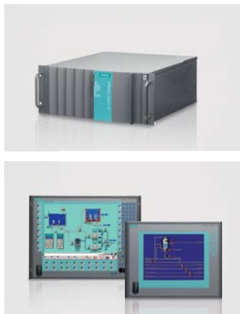
SIMATIC PCs with PROFINET onboard are available in the following designs: Box PC, Rack PC and Panel PC
