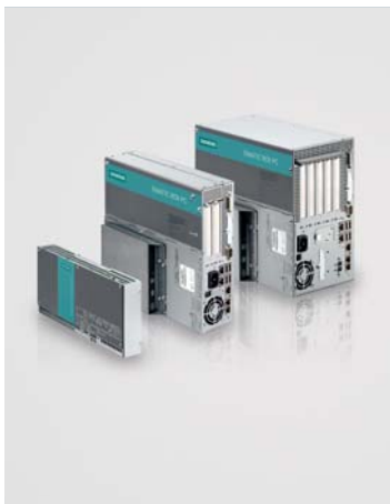
SIMATIC PCs with PROFINET onboard are available in the following designs: Box PC, Rack PC and Panel PC
